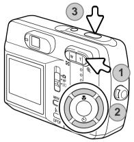
With the image to be magnified displayed, press the right side of the zoom lever (1) to enlarge. Pressing the right side of the zoom lever increases the image magnification. Pressing the left side of the zoom lever decreases the image magnification.
