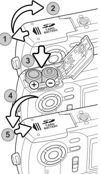
Open the battery-chamber door on the bottom of the camera by sliding the door toward the side of the camera (1) to release the safety catch; the door can then be opened (2).
