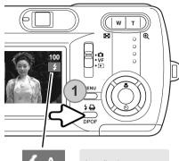
frame advance recording mode. To select the flash mode, press the flash-mode button (1) on the back of the camera until the desired mode is displayed. The active flash mode is displayed near the top right corner of the LCD monitor. The flash mode setting will remain until it is changed. While the flash is charging, the shutter cannot be released.
