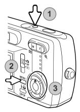
Turn the camera on (1) and press the menu button to display the function menu (2). Use the up/down and left/right keys of the controller to highlight the setup mode at the top line of the menu options (3).
