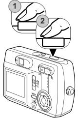
Press the shutter-release button partway down (1) to lock the focus and exposure.
