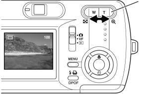
The zoom lens is operated by the zoom lever. Pressing the right side (T) will zoom in to the telephoto position of the lens. Pressing the left side (W) will zoom out to the wide-angle position. The optical zoom position is indicated by the scale at the bottom of the LCD monitor.
