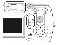
6. Slide the mode switch to the playback position (1) and turn on the camera to initiate the USB connection. While the camera is connected to a computer, the camera's monitor will not activate, and the green indicator lamp will glow steadily.
