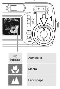
To set the focus mode, simply press the up key of the controller (1) until the desired mode is displayed. The focus mode setting will remain in the recording mode you set until it is changed.
